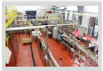
The following day the entire system was coated with a Flowfresh SR sealer topcoat, to provide an outstanding chemical resistant, cementitious urethane floor, ideal for wet processing zones in food and beverage manufacturing facilities because it contains Polygiene, an antimicrobial agent that inhibits the growth of 99.9% of bacteria, making it ultra hygienic.
